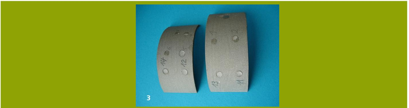
1 Carbon fiber tube with ceramic coating.
