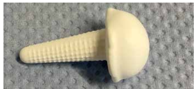
Slip-cast patient-specific implant made of ATZ.
