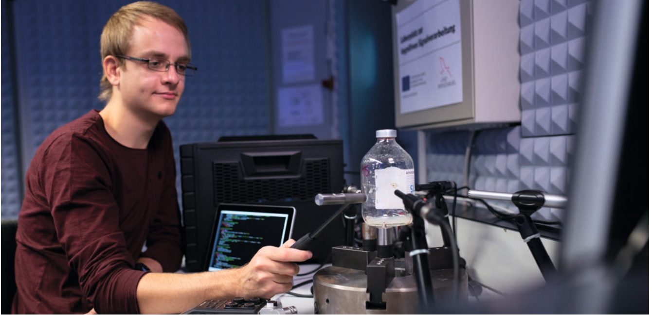
Crack testing of glass bottles using acoustic resonance analysis.
