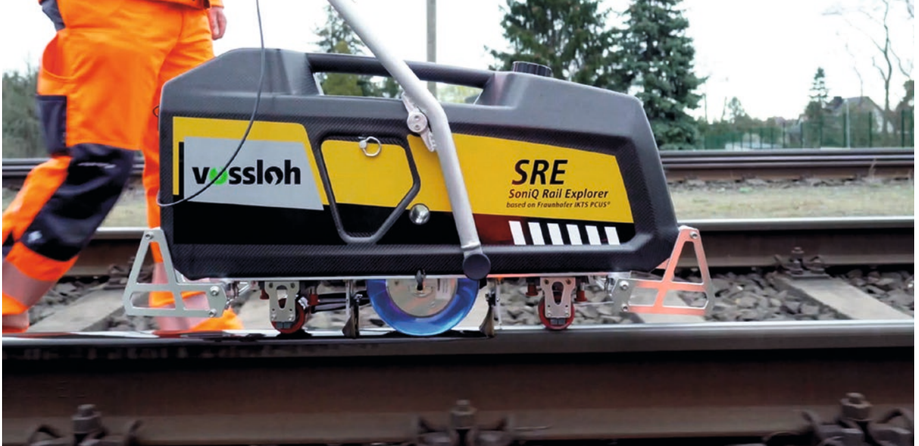
The SoniQ Rail Explorer for mobile ultrasonic rail inspection demonstrates the range of services offered by Fraunhofer IKTS, from test concepts to sensors, electronics, software and robust, industrially compatible testing devices (source: Vossloh Rail Services).
