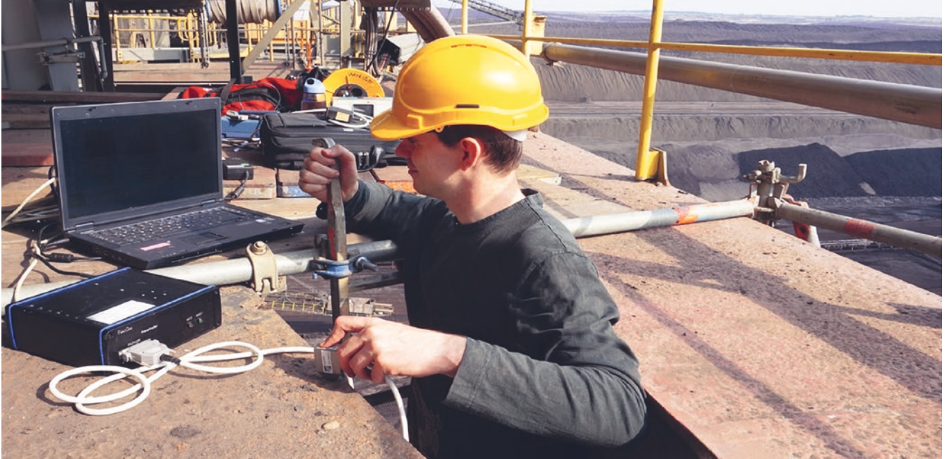
Testing weld seams on frame structures by means of micromagnetic Barkhausen noise.
