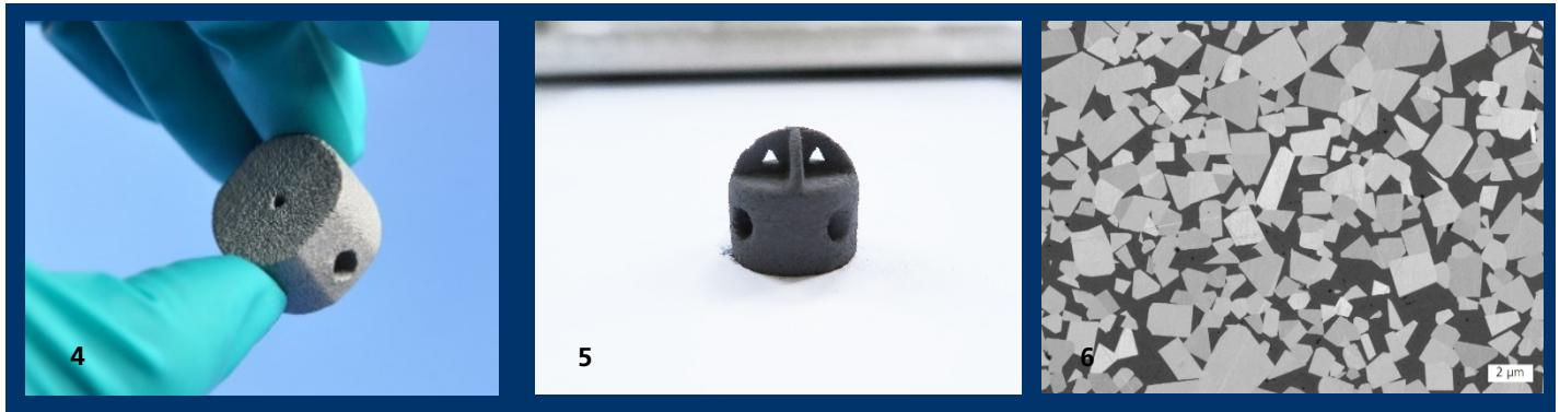
1 *Structure of a 3D printed hardmetal with the composition of WC-12Co (FESEM).*
