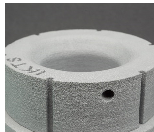
Sintered drawing nozzle with helixshaped cooling channel.
