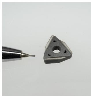
*FFF printed hardmetal insert with chip breaker geometry.*
