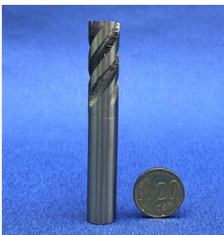
*FFF printed, sintered and grinded WC-10 wt% Co end mill.*
