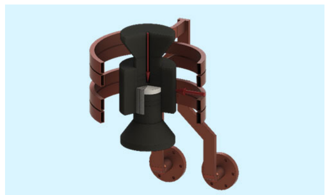
Sectional drawing of graphite tool and induction heating coil.
