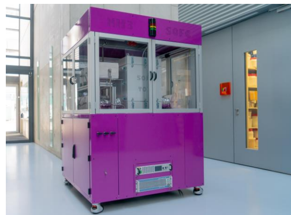
Figure 3: NH 3 – SOFC demonstration plant.
