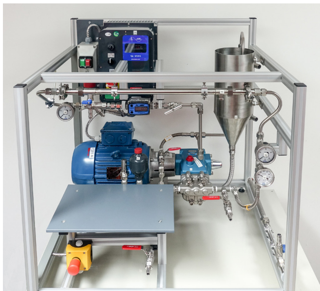
Filtration plant (lab scale), table-top construction, built by Fraunhofer IKTS.
