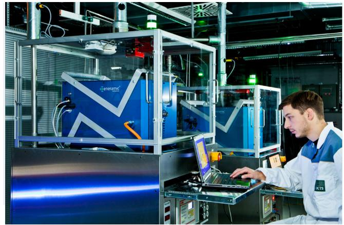
*Fully automated test stand for fuel cells, which can also characterize electrolyzer cells in accordance with the "EU harmonized pro-ocols for testing of low-temperature water electrolysis".*
