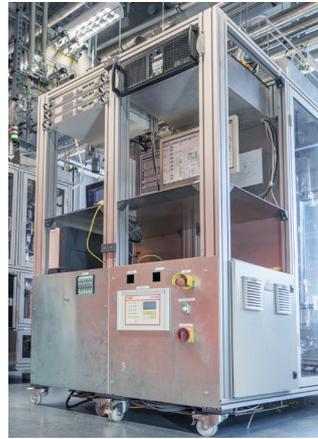
*Plant for coupling of co-electrolysis and Fischer-Tropsch synthesis to produce value-added products.*
