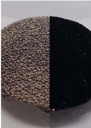
*Ceramic-coated electrode for alkaline energy converters, e.g. as gas diffusion electrode.*
