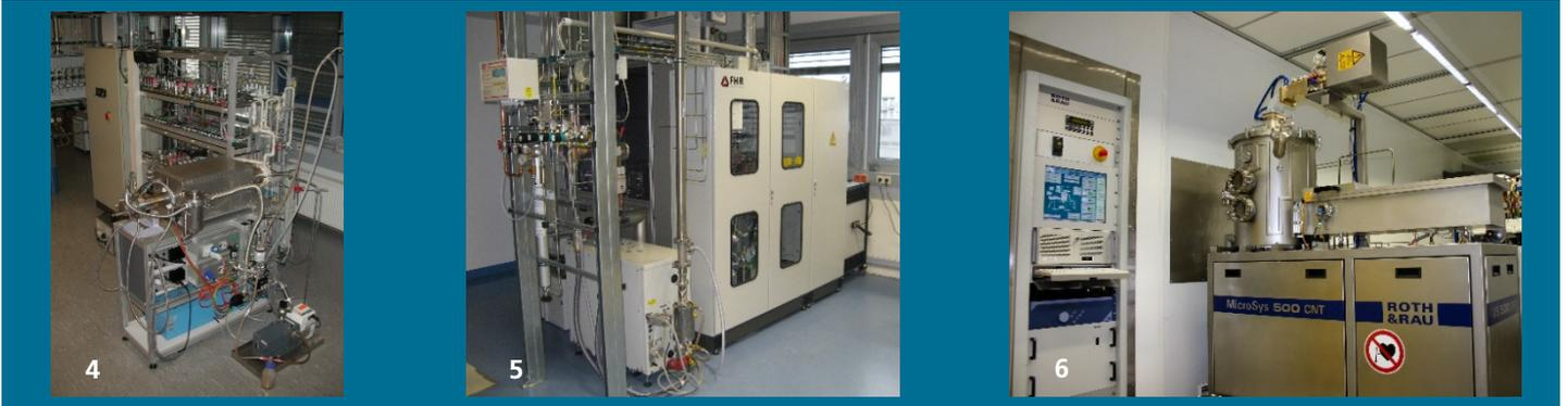
1 Lab-scale coating equipment (CVD, ALD) for batch as well as roll-to-roll-processing.
