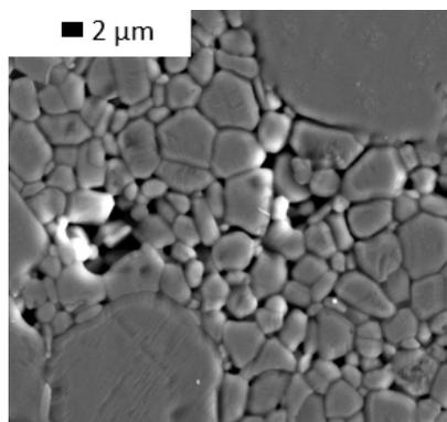
Fig. 2 Microstructure of a Na-β"-alumina electrolyte recorded by SEM.
