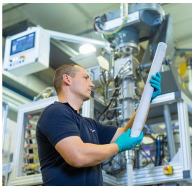
Fig. 3 Electrolyte tube made of Na-β"-alumina before sintering.
