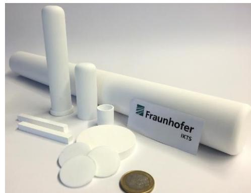
Fig. 4 Different shaped electrolytes made from Na-β"-alumina.
