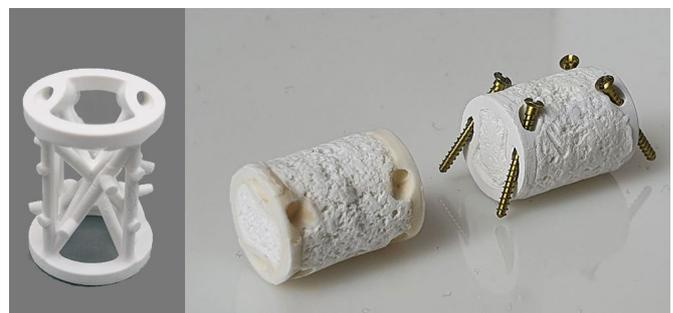
*Hybrid-bone test implant: inner CerAM VPP support (TCP/ZrO<sub>2</sub>; left) and foamed-in Freeze Foam (TCP).*
