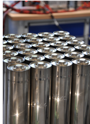
100 Ah battery cells.
