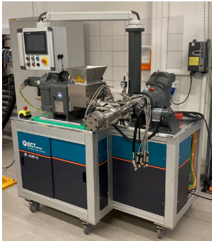
Fig. 1: VAQRS 35 extruder for electrode extrusion.
