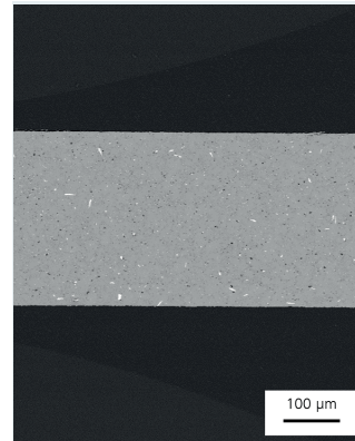
SEM cross section of a sintered tape.
