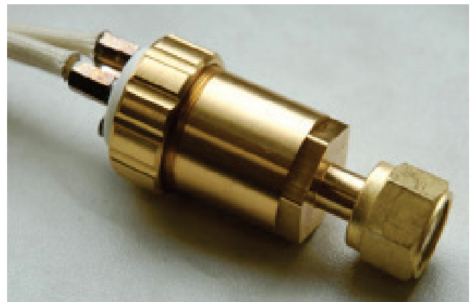
Overall view of the TCSI detector.
