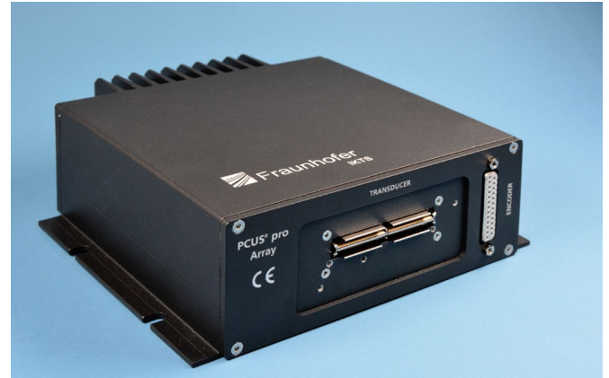
PCUS ® pro Array frontend – front side.
