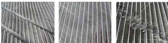
Possible defects during NCF production: Gaps, overlapped tows, fringes.
