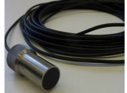
Single element transducer probe for immersion technique till 2 m water.
