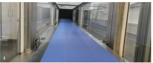
1 Discontinuous casting plant with integrated UV modules at the tape casting facility of Fraunhofer IKTS in Hermsdorf.
