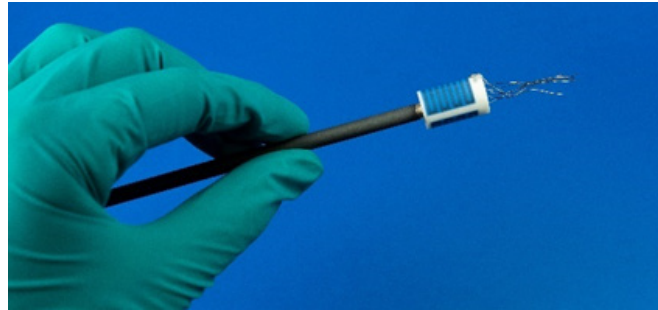
Additively manufactured reference temperature point for inclusion of ceramic thermocouples with integrated heaters.
