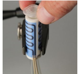
Functionalized PCR test module with integrated heating and cooling structures.
