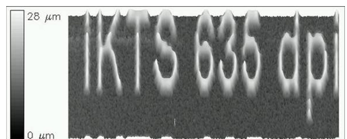
Inkjet printing of a Ag ink on Si wafer.
