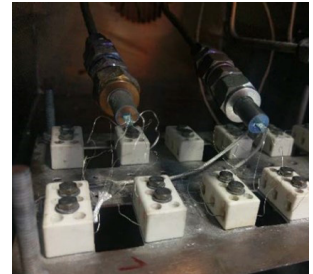
Automated high-temperature pressure test stand.
