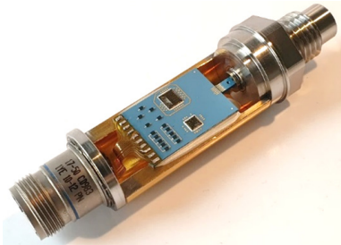
Pressure/temperature combination sensor with integrated electronics.
