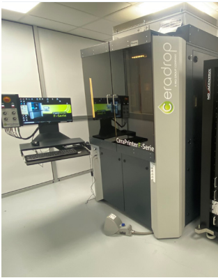
Multi-material printer with inline drying and sintering.
