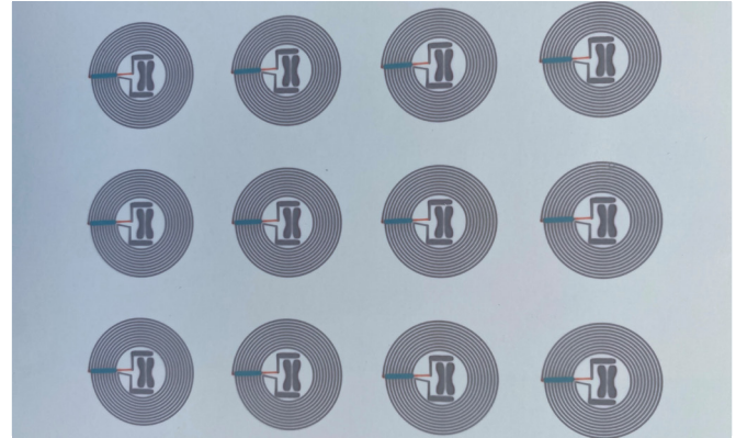
Printed functional layers in electronics: coil array in inkjet multilayer printing (in cooperation with J.A.M.E.S GmbH).
