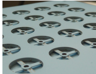
Fabrication in multiple panels: 25 sensors per 4-inch substrate.
