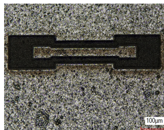
Modulated attenuation constant of S-parameter measuring. Laser-structured CPWG on LTCC.
