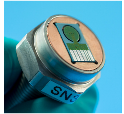
Packaging of LTCC pressure sensor in metallic pressure connection.
