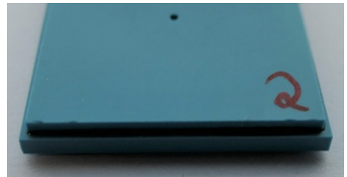
Joint "normally open" valve (top view).
