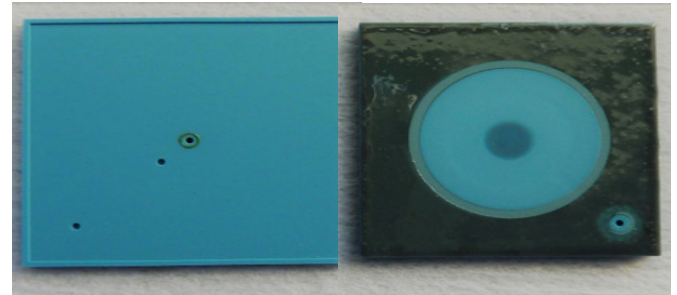
Base body (left) and membrane body (right) of a "normally closed" valve.
