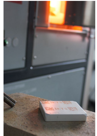
Temperature-stable marking of ceramics after 1,300 °C.
