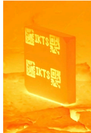
Temperature-stable marking of ceramics at approx. 1,100 °C.
