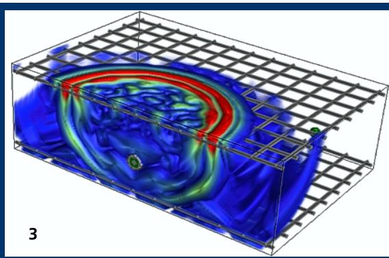
1 Sound field of an ultrasonic angle-beam probe.
