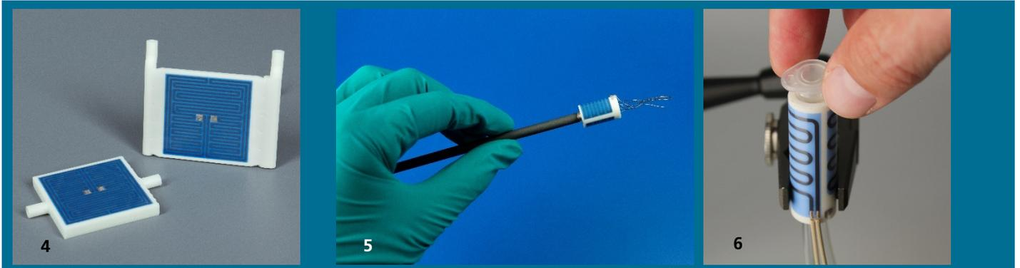
4 Additively manufactured ceramic temperature cycler with integrated water cooling.
