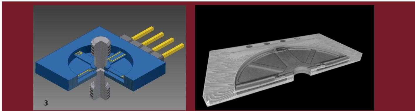
1 *LTCC based miniaturized force sensors for three force ranges.*
