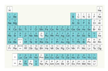
Fig. 1: Elements that could be analyzed by ICP-OES (blue).
