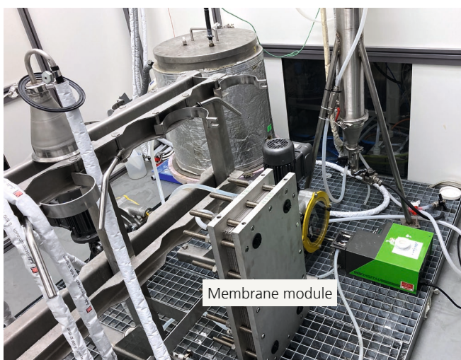
Fig. 1: Pervaporation system with integrated MMM module for hydrophobic EtOH separation (Fraunhofer IKTS).
