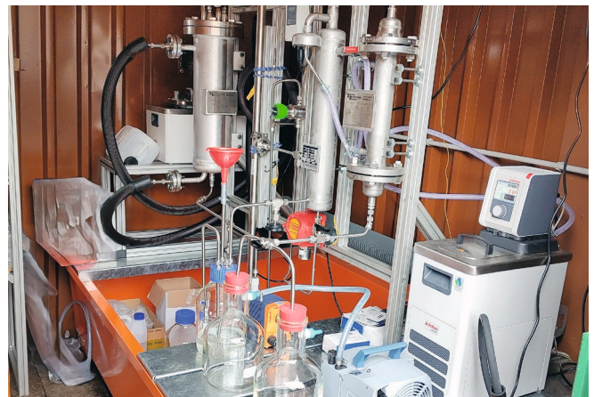
Fig. 2: Unit for water separation using hydrophilic membranes for ethanol absolutization (Fraunhofer IKTS).
