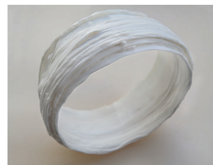
Fig. 2: Wound mold with microchannel structure.
