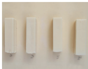
Fig. 1: Formed components with microchannel structure (from slip casting).
