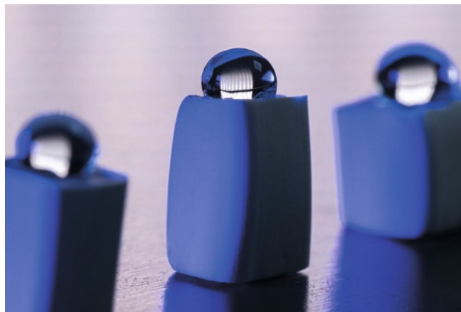
Figure 1: Ceramic adsorbers for the removal of micropollutants (source: Jens Meyer, Friedrich Schiller University Jena).
