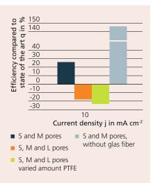
Electrode performance vs. standard electrodes (GDE) for alkaline water electrolysis.
