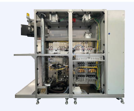
Multifunctional gas phase system (operation at up to 650 °C), under construction, for external use.
