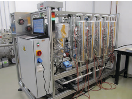
Gas separation system, for external use.
