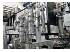
A pyrolysis rotary kiln is used for the upscaling of pyrolysis processes. The liquid products, containing the valuable chemical compounds, are obtained in a condensation unit.
