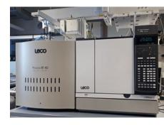
Complex mixtures of organic compounds, such as synthetic fuels or pyrolysis oils from plastics, are analyzed using comprehensive gas chromatography mass spectrometry.
