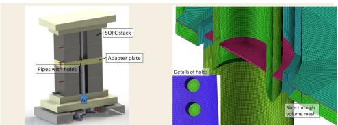
Geometry of hotbox with 8 SOFC stacks. Detail of mesh (16 Mio. control volumes).
