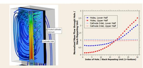
Streamlines (coloured by flow velocity) in the upper half of the hotbox. Mass flow distribution per hole / stack repeating unit.
