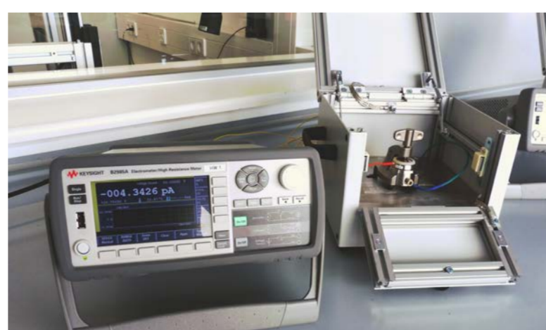
Pic 8: Keithley high precision electrometer with faraday cage and EI-Cell.
