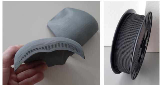
Scaled double walled SSiC body armor manufactured by Fused Filament Fabrication (CerAM FFF). Ceramic filament.
