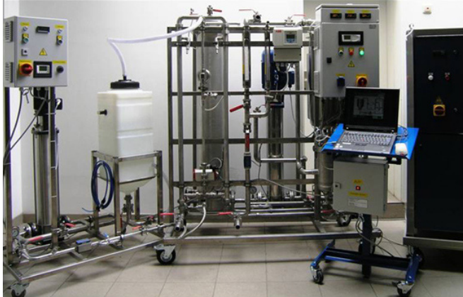
Mobile membrane plant VSA IKTS with membrane areas from 0.1 m 2 to 2.6 m 2 , with PID controller, back-flush unit, data logger.
