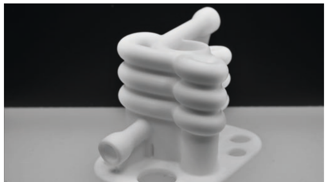
Figure 2: Front view of a Tesla valve with inlet for counter-current in the foreground.
