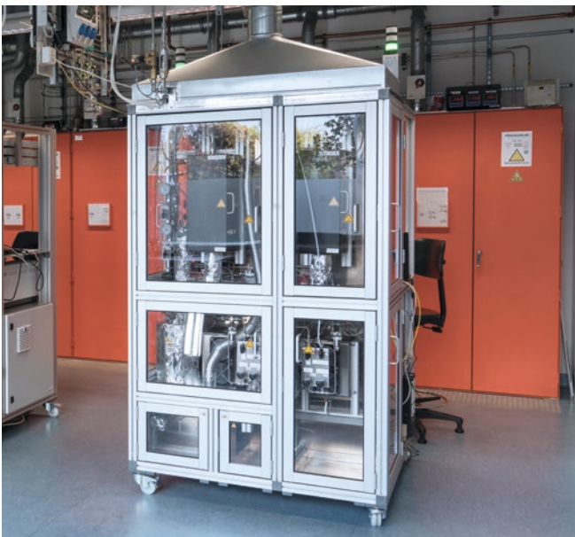
Figure 1: Test plant for the performance of degradation tests.
