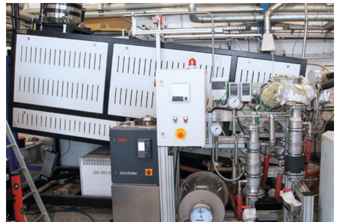
Figure 1: Pyrolysis rotary kiln on a pilot-plant scale with a specially designed and built condensation system in the foreground.
