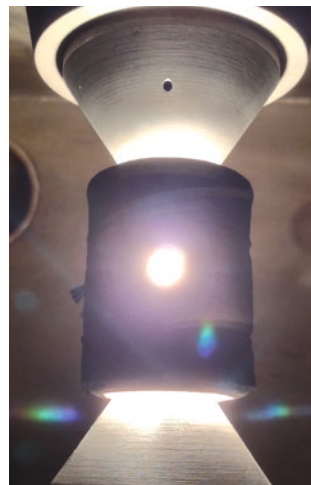
Figure 2: Tool with graphite felt cover during the FAST process.
